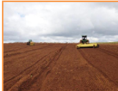
Rocks up to 1.5 feet can be handled with a Rock Rake. Surface rocks are winrowed from two sides and picked up by the Rock Picker.
